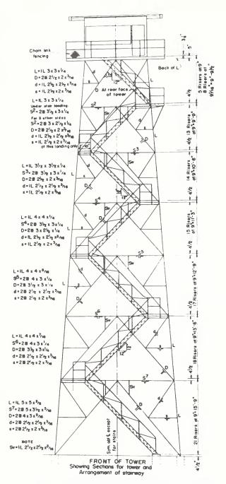
2 angle sections shall have long or short legs back to back as shawn. ¬resections to be field bolted with ring fillers at about 2 ft intervals. Balts in tower members 3/4\* ∉ except for connections as noted on detail Gusset plates 5/6\* for tower members. Working lines as shown above are gage lines except as shown ar noted.
